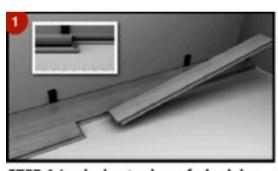
STEP 1:Lock short edge of plank by inserting tongue into groove
