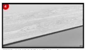
STEP 4:IMPORTANT! Use hammer or strike hard with your hand, make sure tongue into the groove and clic perfectly
