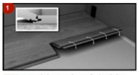
STEP 1:Lock long edge of plank by inserting tongue into groove at an angle and drop in place.
