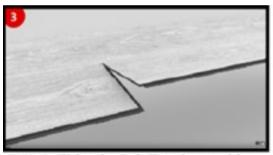
STEP 3:Slide plank follow long side toward until the short side tongue just touches the groove
