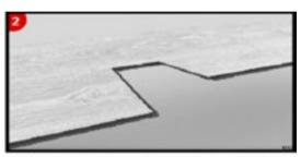
STEP 2:Make sure long edge of plank tongue into groove at an angle click
